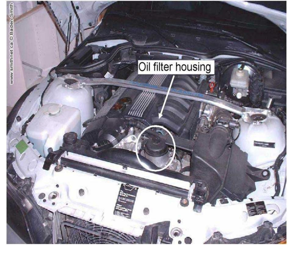
Step 20. Remove the housing and the filter insert. Place a cloth under the filter as you remove it to prevent any oil from dripping on the engine. Place it on a piece of paper.
