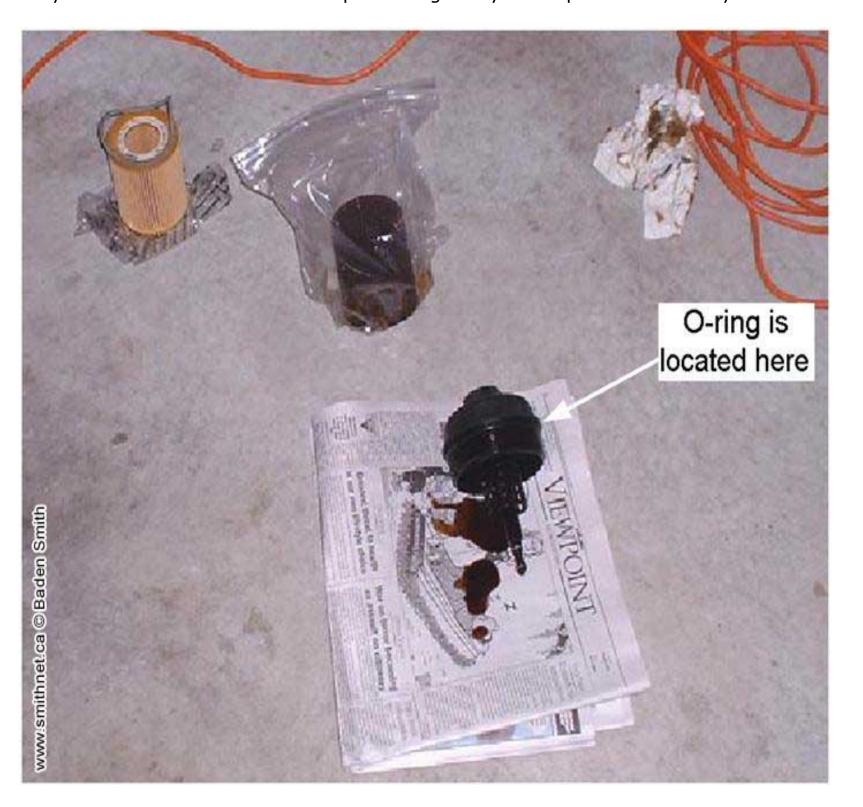
Step 24. Remove the old O-ring on the filter housing and discard.
